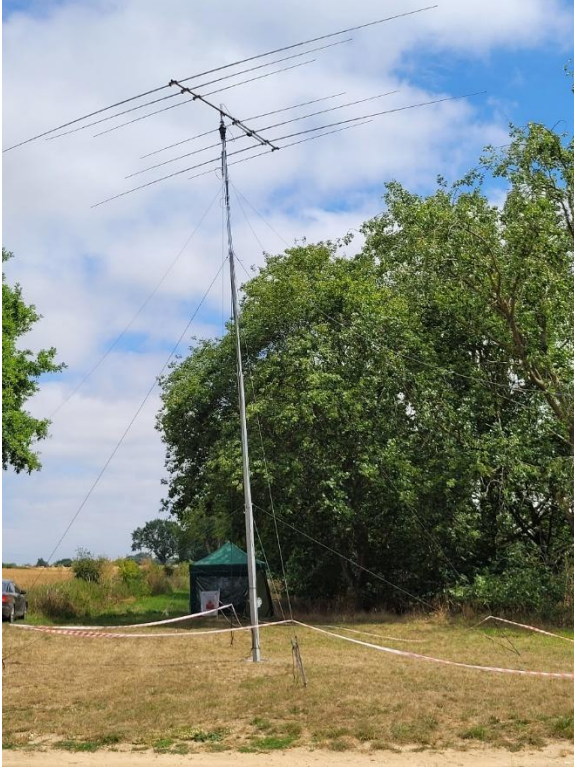
Antennas at Site 805. 7-element trapless tribander at about 30' and inverted vees for 80 and 40.
